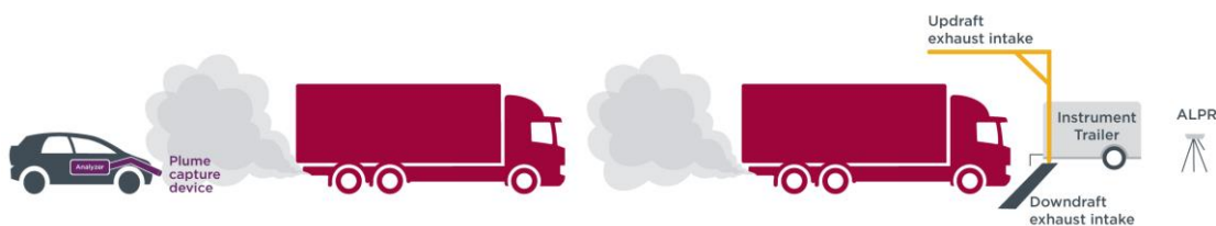
Figure 3a: Schematic setup of a plume chaser installed in vehicle measuring the exhaust emissions from the truck in front
